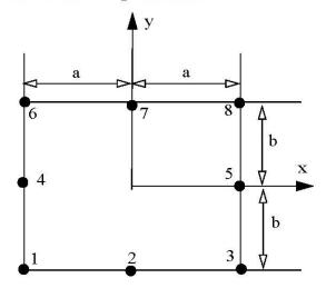
• When internal nodes are eliminated care has to be exercised to ensure the mesh from such elements will converge.
