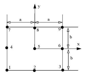
• The stiffness (row and column) related to node 5 is known at element level and as rows and columns of other elements do not add to it.
