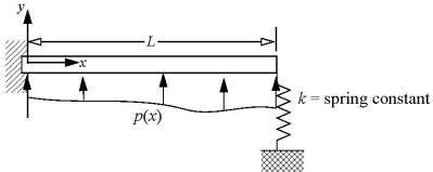
Obtain the BVP for the beam shown above using variational methods.
