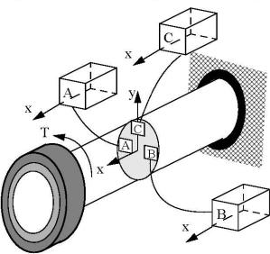
C5.4 Determine the internal torque in the shaft below by making imaginary cuts and drawing free body diagrams.
