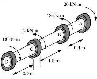
C5.6 A solid circular steel ( $G_s = 12,000 \text{ ksi}$ ) shaft BC is securely attached to two hollow steel shafts AB and CD as shown. Determine: (a) the angle of rotation of section at D with respect to section at A. (b) the maximum torsional shear stress in the shaft (c) the torsional shear stress at point E and show it on a stress cube. Point E is on the inside bottom surface of CD.
