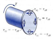
C5.3 Determine the direction of shear stress at points A and B (a) by inspection, and (b) by using the sign convention for internal torque and the subscripts. Report your answer as a positive or negative  $\tau_{xy}$ .
