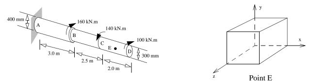
3 (a) Draw the shear force and bending moment diagram for the beam and loading shown. Clearly mark the numerical values and write the nature of the curve (convex, concave, linear).
