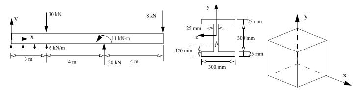
ANSWERS<br/>1c $\sigma_A = \text{Compression}$  $\sigma_B = \text{Tension}$  $\sigma_C = \text{Tension}$  $\sigma_D = \text{Compression}$ 1d=FALSE1e=TRUE(1f)  $M_{AB} = -\left(\frac{wx^3}{6L}\right)$ 2.  $\tau_{max} = 25.8 \text{ ksi}$  $\phi_B = 0.0516 \text{ rads CCW}$ 3.  $(\sigma_{xx})_A = 1.94\text{MPa(C)}$  $(\tau_{xy})_A = -1.03\text{MPa}$
