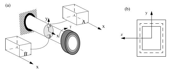
(b) Sketch the direction of the shear flow along the center-line on the thin cross-sections shown, assuming a positive shear force  $V_v$
