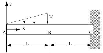
(g) In the beam shown above the internal bending moment in segment BC is:  $M_{BC} = \frac{wL}{6}(3x-2L)$ . Assuming EI is
