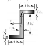
(iii) The internal bending moments on the cross section shown above were determined to be  $M_y = -20 \ kN - m$  and  $M_z = -25 \ kN - m$ . Determine (a) the orientation of the neutral axis and (b) the maximum bending normal stress.
