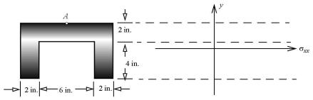
(ii) Determine the three second area moment of inertias  $I_{yy}$ ,  $I_{zz}$ , and  $I_{yz}$  for the cross-section shown.
