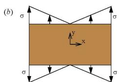
Fourth order polynomial  $\psi = \frac{a_4}{12}x^4 + \frac{b_4}{6}x^3y + \frac{c_4}{2}x^2y^2 + \frac{d_4}{6}xy^3 + \frac{e_4}{12}y^4$
