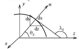
The stress function  $\psi$  must be constant on the boundary of the cross-section of the non-circular shaft
