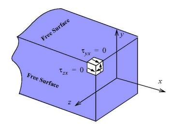
There is a transition region near towards the edge of  $y = \pm b/2$  where the torsional shear stress  $\tau_{xz}$ , which we neglected is nonzero.
