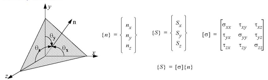
$n_x$ ,  $n_y$  and  $n_z$  -- direction cosines of the unit normal to the surface in the x, y, and z direction.
