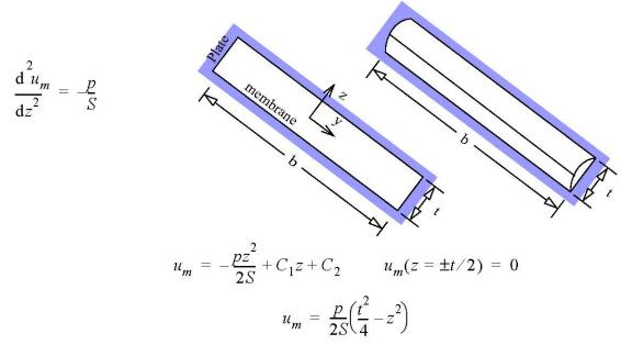
• At  $y = \pm b/2$  the approximate membrane deflected shape is incorrect.
