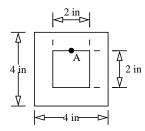
A steel  $E_{steel}$  = 200 GPa strip is attached to a aluminum  $E_{Al}$  = 70 GPa beam to form a composite cantilever 3. beam as shown. Determine the maximum bending normal and shear stress in steel and aluminum.
