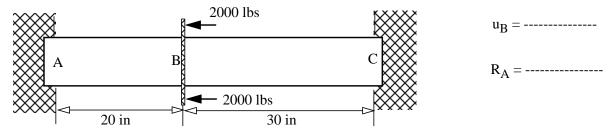
3. (a) For the beam shown determine a kinematically admissible displacement function using coordinate shown.
