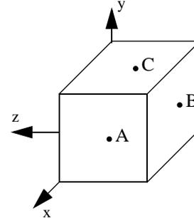
(b & c) The normal stresses at a point were found to be  $\sigma_{xx} = 200 \text{ MPa (T)}$ ,  $\sigma_{yy} = 100 \text{ MPa (T)}$ . The material has a modulus of elasticity of  $E = 200 \text{ GPa}$  and Poisson's ratio  $\nu = 0.25$ .
