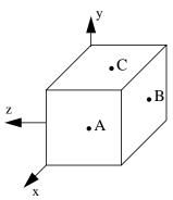
(b) Draw the shear stress due to torsion on the stress cubes at points A and B. Is the shear stress positive or negative? Circle the appropriate answers
